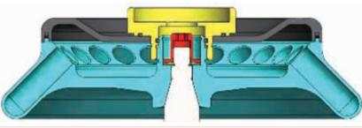
DLAB rotors are manufactured from militaryindustrial grade aluminum alloy with high mechanical strength for precise running and safety (excludes D2012 plus rotor)
